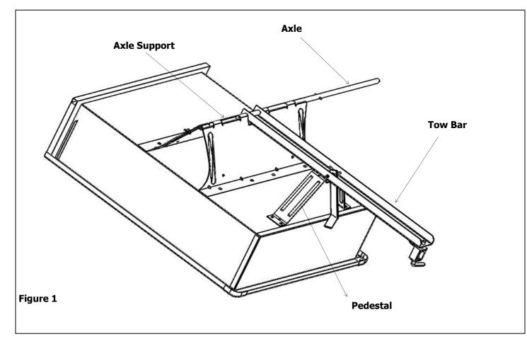
2. Center the Axle in the Axle Support then place one 3/4" Flat Washer on each side of the Axle next to the Axle Support. Place one Wheel on each side of the Axle and one more 3/4" Flat Washers on the outside of each Wheel. See Figure 2.
