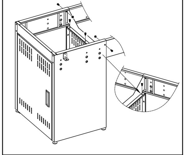
11. Attach the Main Table (P) onto the box assembled in step 10 with 6 M6X12 Bolts, keep the assembly holes aligned at the holes in the bracket.
