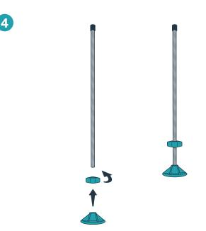
Screw a large wingnut onto the uncapped end of each threaded rod. Twist a round cap tightly onto the same end of each threaded rod.
