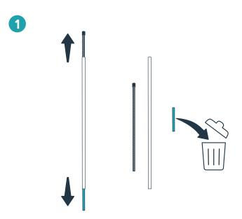
Remove the threaded rod and short, black plastic spacer from inside each of the two straight tubes. Discard the two plastic spacers.
