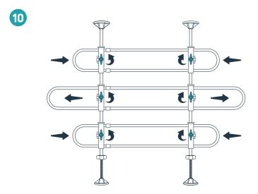
You can extend each tube to the left, to the right, or to both sides to fit your vehicle. Loosen the wingnuts on the clamps to extend or shorten each oval tube. When each oval tube is the width you want, tighten the wingnuts on the clamps.
