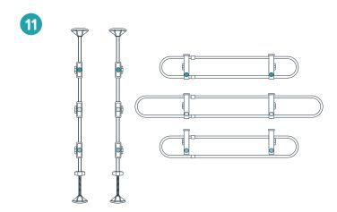
You can use the included stickers to color-code the pieces to make setup quick and easy each time. Match each pair of oval tube clamps with the corresponding pair of mounting brackets.
