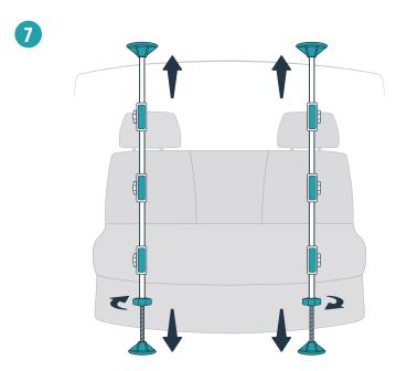
Insert a threaded rod into each hollow tube to form a pair of upright supports. Stand them up with the round bottom caps on the floor, spaced evenly across the width of your vehicle. Rotate each large wingnut to adjust the height until each oval top cap is pressed firmly into the ceiling. Both upright supports should now stand securely on their own.
