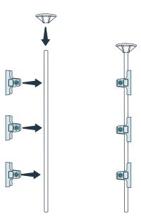
Push an oval cap firmly onto one end of each straight tube. Slip three mounting brackets onto one straight tube with the hexagonal holes all facing the same side. Slip three mounting brackets onto the other straight tube with the hexagonal holes all facing the opposite side, so the two tubes mirror each other.
