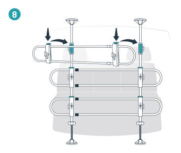
Mount each oval tube onto the upright supports. To snap each pair of clamps into place, press and hold the blue buttons, slide the clamps down onto the rectangular slots on the mounting brackets and release the blue buttons.
