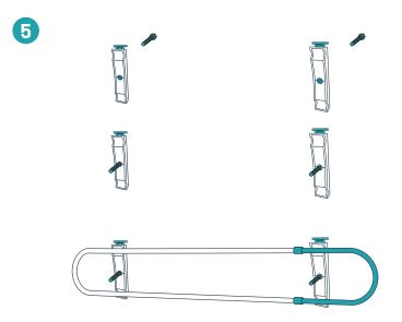
Insert a long bolt through each of the clamp halves with blue buttons, fitting the bolt head into the hexagonal hole. Position two of these clamp halves with the blue buttons facing the same direction, then set an extendable oval tube across them. Make sure one clamp half is on the extendable (thinner) section of the oval tube.
