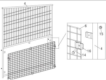
• The Moveable Mesh (6) is pre-assembled with Side Panel II (4). It can be taken-off if customer needs an extra opening.
