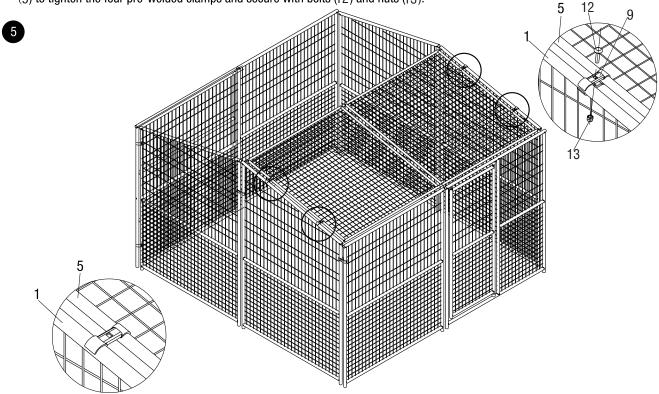
• Repeat the above procedure to finish attaching the half roof.
