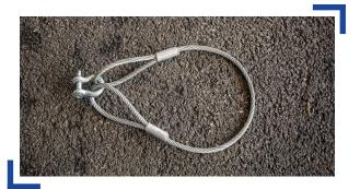
Take small cable and run through the loop of one end of the long cable.
