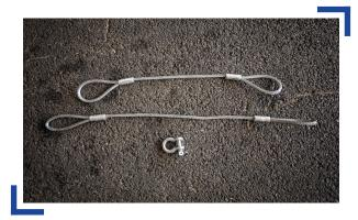
Using clevis, connect both ends of the short cable.
