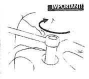
8. This step is critical to the performance of your Zigzag Car! Use a 17mm socket wrench to tighten the nut in the steering column as tight as possible. You can also use the included hex key tool.
