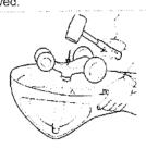
5. Strike the base of the front wheel assembly with a rubber mallet. The metal bearing should be seated securely in the body.
