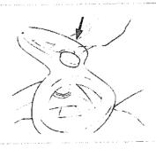
9. Push the cap onto the steering wheel...
