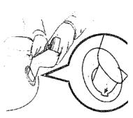
1. Fit the notch on each rear wheel housing into the body. Push the wheels in at a 45 degree angle. When installed correctly, the rear wheels flare out from the body. Once locked into place, the
