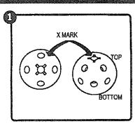
Locate the X marks on top and bottom of your connector.
