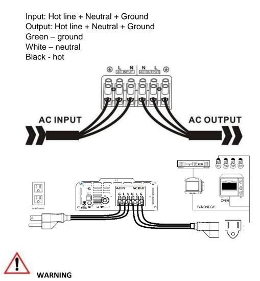
The output voltage of this unit must never be connected in its input AC terminal, overload or damage may result. Always press power button to ON position before plugging in any appliance.
