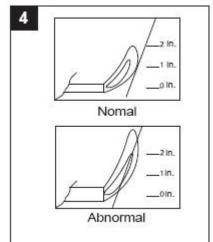
flames should not be yellow or produce thick black smoke, indicating an obstruction of airflow through the burners. The flame should be blue with straight yellow tops. If excessive yellow flame is detected, turn off heater and consult "Troubleshooting" on page 19.
