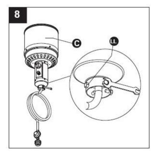
9. Insert hose of head assembly (C) into post (J). Secure head assembly (C) to post (J) with stainless steel bolts (LL).
