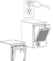
**Step 1:** Make sure the unit is unplugged before installing, removing any filters or maintaining the unit in any way, to prevent electric shock.
