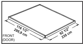
Note: Finished Slab dimensions, with lumber removed.
