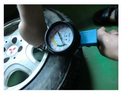
1. By aligning the inflatable rod with the valve core of the tire, it can measure the pressure for the tire. And the tire can be deflated when the trigger is pressed half.
