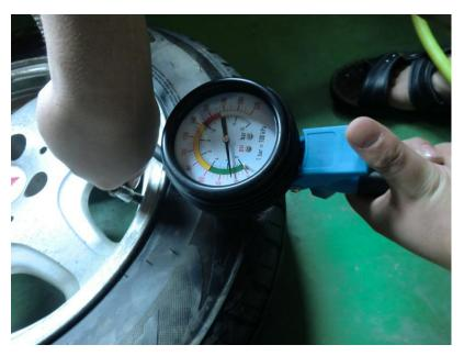
2.After connecting the air compressor, it can inflate of tire when the trigger is pressed to the end.
