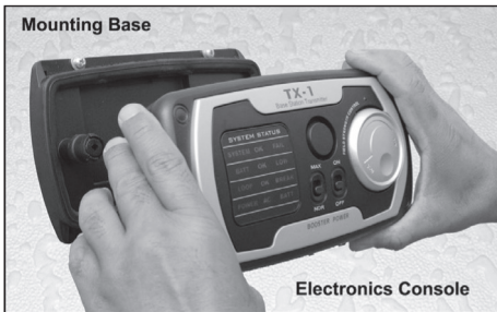
A. Separate Mounting Base From Electronics Console.
