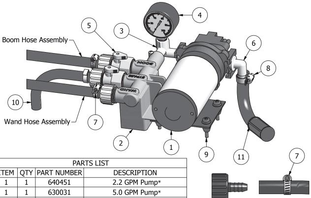
**ITEM** Manifold Body Elbow (2.2 pumps) Elbow (5.0 pumps) Gauge 0-100 PSI Inline Valve QD EL 12 5/8" Hose Clamp 1/2" Hose Clamp 10-24 x 1.25 Screw Relief Hose Assembly Suction Hose Assembly
