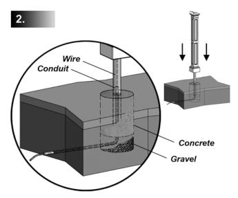
For hard-wired installations thread UF rated wire through the mounting post and into the conduit. The conduit can be buried beside the post or directly in the center of the concrete footing leaving 6 inches exposed above ground. Outdoor wiring should be buried in conduit 18 to 24 inches below ground. Once the concrete has cured, slide the decorative sleeve over the mounting post.
