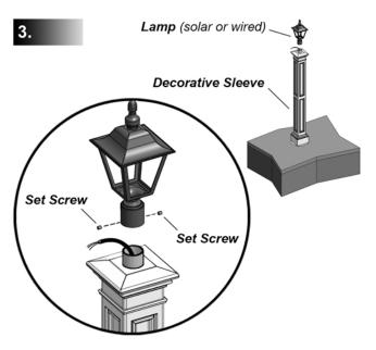
The decorative sleeve should sit flush on the ground leaving two inches of the mounting post exposed at the top. Connect the wiring and secure the lamp to the post. For solar lights simply secure the lamp to the post.
