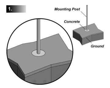
For solar lamp installations simply dig a hole approximately 15 inches deep and set the mounting post in place leaving 74 inches above ground. Fill in the hole with concrete and allow time to cure. For added stability dig a deeper hole and add 6 inches of gravel. This improves drainage and helps prevent heaving from frost.
