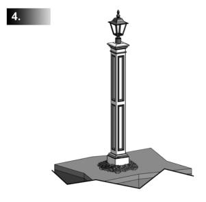
Remember to leave extra wire to reach the circuit-breaker panel inside the house. All outdoor wiring should be installed according to local electrical codes and inspected by a licensed electrician. To complete the installation you can back fill dirt around the base of the lamp post.
