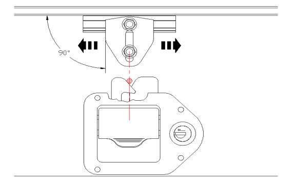
2) When the striker pin is correctly centered, tighten top bolt to set the location.
