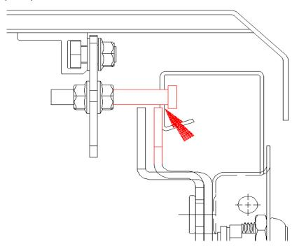
4) Tighten the pin in the lowest location, and close the lid. If the lid is able to move up and down when latched, the latch pin needs adjusted. Adjust the pin up the approximate amount the lid is able to move and retighten. Repeat as necessary.
