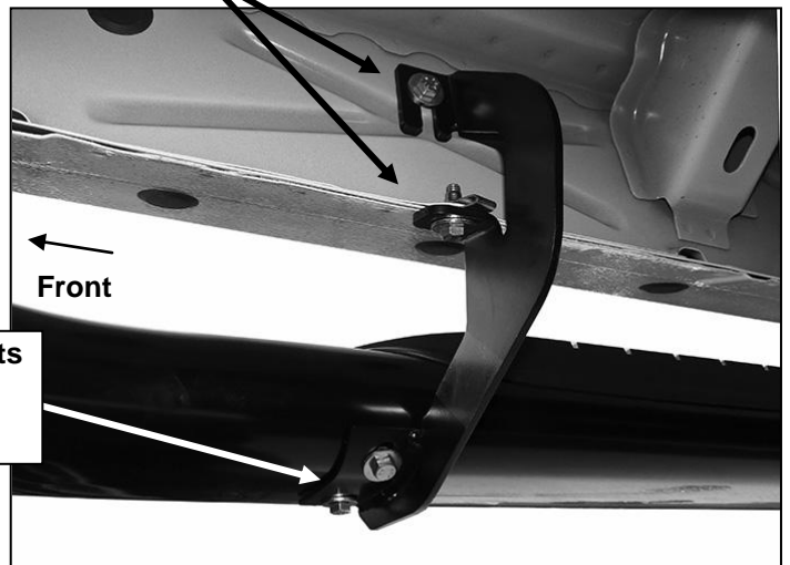
(Fig 9) Passenger side front Bracket installation
