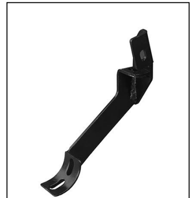
(Fig 16) Passenger/right Front Lower Bracket (all models)
