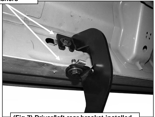
(Fig 7) Driver/left rear bracket installed
