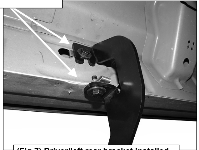
(Fig 7) Driver/left rear bracket installed
