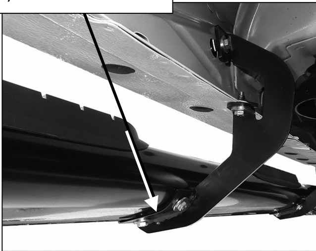
(Fig 17) Passenger side installation pictured
