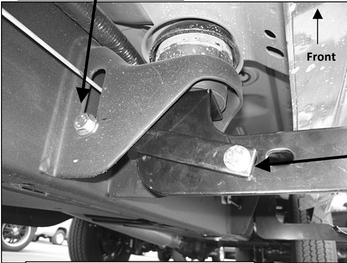
(Fig 6) 1500 Model Center Support Bracket Installation Pictured
