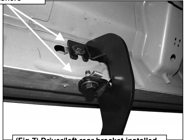
(Fig 7) Driver/left rear bracket installed
