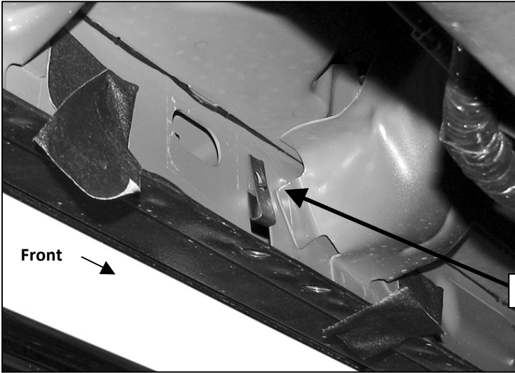
(Fig 4) Driver side-center Mounting Bracket location
