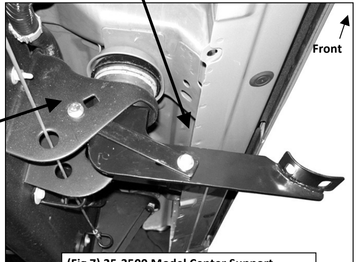
(Fig 7) 25-3500 Model Center Support Bracket Installation Pictured
