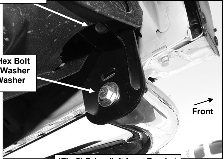
(Fig 5) Driver/left front Bracket
