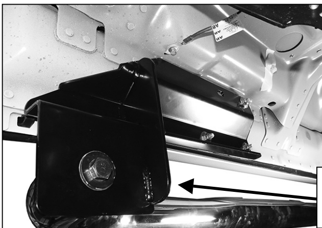
(Fig 5) Passenger side front Bracket installation
