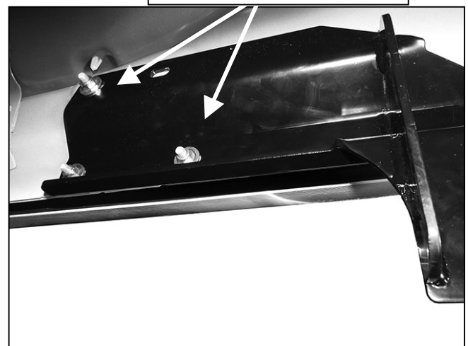
(Fig 4) Passenger side rear Bracket installation
