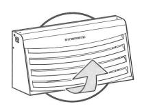
Install **IND35L** by offering the product up to the wall and marking the three fixing centers. Then drill holes and fit the supplied wall plugs and screws. (For specialist wall surfaces such as plasterboard, appropriate wall plugs should be used.) Then hand the product onto the mounting screws.
