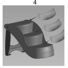
Remove the paper backing. Align the tread with the designated area on the step and press into position. Repeat until all steps are covered.
