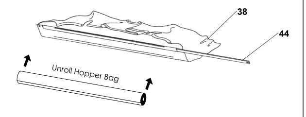
First, place bottom frame assembly into bottom of Hopper Bag (38).
