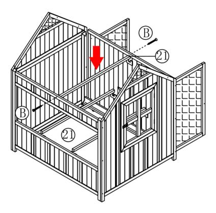
Step 5: Attach the right and left nesting panels (8) using screws (B)\*6pcs as shown.
