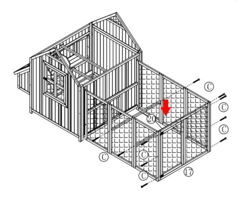
Step 12: Attach the run left cover panel (18) and the run right cover panel (19) to the run side panels using screws(C)\*14pcs as shown.
