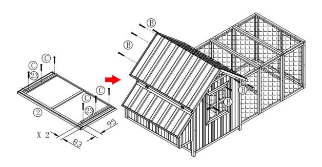
Step 14: Attach the roof cap (1) using screws (C)\*4pcs as shown.
