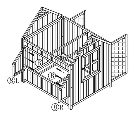
Step 6: Place the nesting floor (9) inside the nesting box. And then install the nesting box divider (22) as shown.
