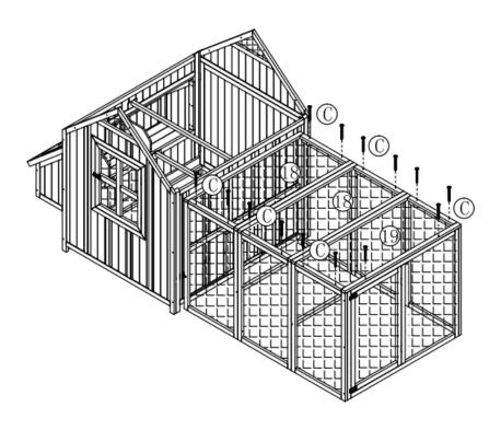
Step 13: Place the support bar (23) to the top roof panels (2) using screws (C)\*12pcs as shown. Then place the roof on the top of coop and secure in place using screws (B)\*8pcs.
