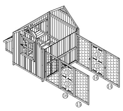
Step 11: Attach the right run panel (17) to the run side panels using screws (C)\*6pcs as shown.
