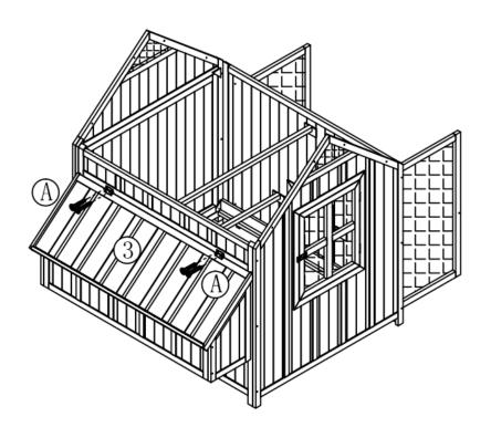
Step 9: Open the nesting roof and attach the support arms (F) to the nesting roof panels using screws (A)\*8pcs.
