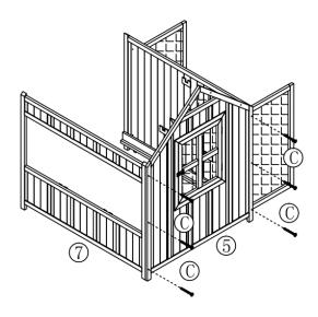
Step 3: Attach the back coop panel (4) to the left and right coop panel using screws (C)\*6pcs as shown.
