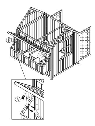
Step 10: Attach the run side panels (14) (15) (16) to each other using screws (D)\* 12pcs as shown.
