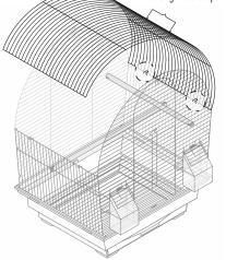
On the remaining side, pull the roof down taut and catch the bottom of the roof under the wire loops along the side panel.
