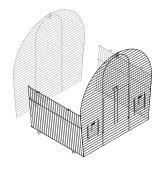
Start at the bottom. Pull the bottom wire hook from the side panel onto the outer wire of the back panel.
