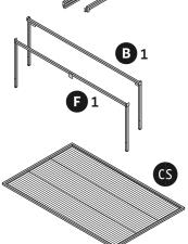
Orient the back legs (B1) with the tray channel backstop facing the back. Attach legs to sides with hex screws in the bracket bottom holes.
