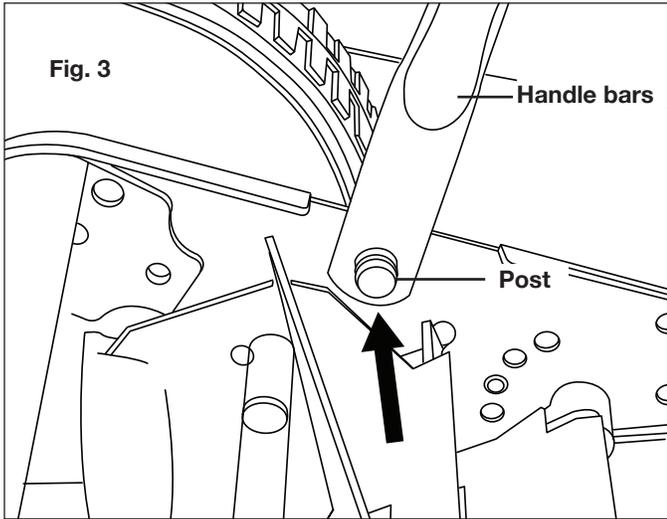
4. Pull both sides of the lower handle bars over the posts on the mower body. Press inward on the handle bars to ensure a secure fit over the posts.
