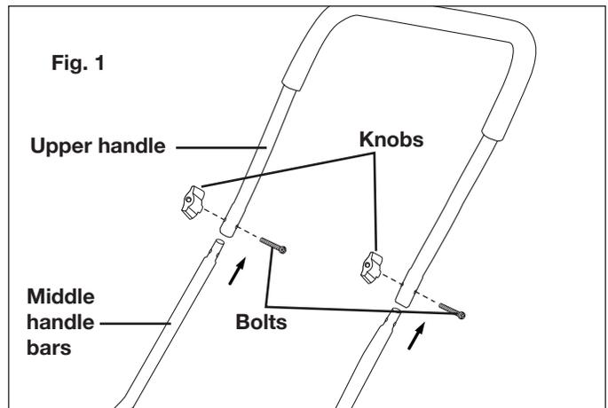
2. Attach the upper and middle handle assembly to the lower handle using the remaining knobs and bolts provided. Tighten the knobs on each side to ensure a secure fit (Fig. 2).
