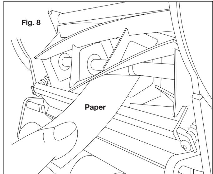
3. All the blades should slice the paper evenly along the entire length of the cutting bar while the reel is turned smoothly.
