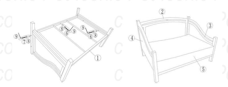
Step One: Insert washers (part 8) into the screws (part 7), and using Allen key (part 9) attach the side panels (part 3 & 4) to the back panel (part 2). Number of screws (part 7) 4 pieces.
