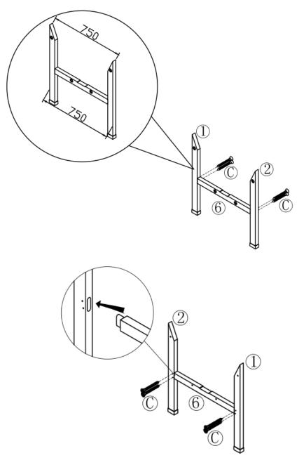
Step 2: Assemble the supports (7) to the middle connector (5). Then assemble the middle post (3 and 4). Attach everything with screws(C) \* 4pcs and screws(B) \* 4pcs as shown.
