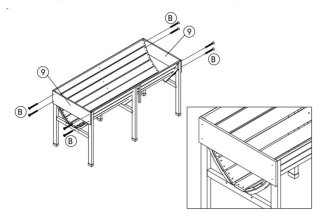
Step 7: Attach the Lower End Panel (10) as shown with screws (B)\*10pcs.
