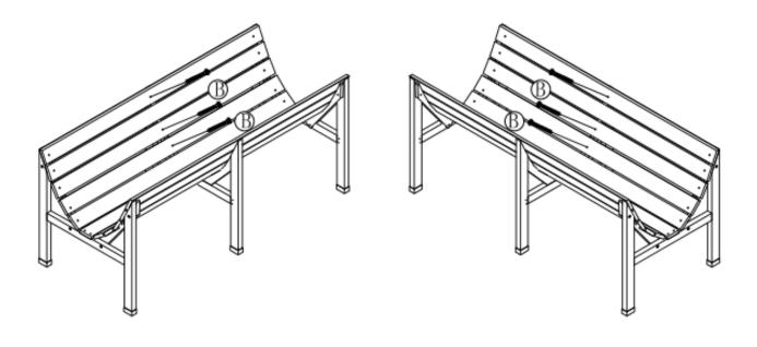
Step 6: Attach the Upper End Panel (9) as shown with screws (B)\*8pcs.
