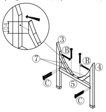
Step 3: Place the Floor Panel (8) as shown, and attach the Floor Panel to the middle connector with screws (B)\*6pcs.
