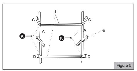
Step 5: Connect Top Leg Frames (C), Lower Leg Frames (D), Support Frames (I) and Side Long Frames (A) by using Bolt and Washer Sets (K) as shown in Figure 5.
