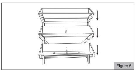
Step 6: Place assembly from Figure 3 into assembly from Figure 5 as shown in Figure 6.
