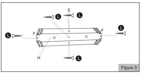
Step 3: Connect Middle Braces (E), Side Braces (F) and Bottom Frames (H) by using screws (L) as shown in Figure 3. (Repeat this two times)
