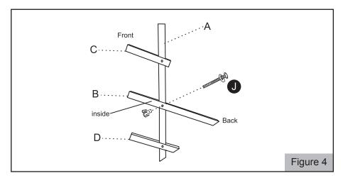
Step 4: Connect Middle Leg Frames (B) and Side Long Frames (A) by using Bolt Sets (J) as shown in Figure 4. (Repeat this on other side)
