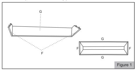
Step 1: Inserted Side Braces (F) into Side Frames (G) faces inside as shown in Figure 1.
