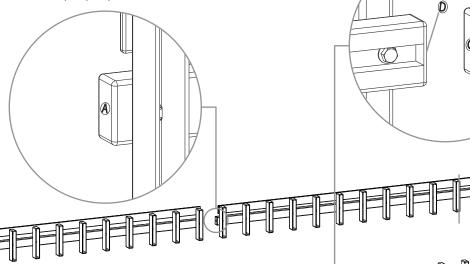
When assembling, match louver bar A with B, and C with D. There will be 3 A's, 3 B's, 3 C's, and 3 D's as shown below:
