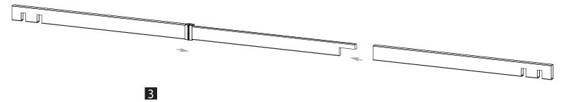
Glue and attach the Decorative End Caps onto the ends as shown.
