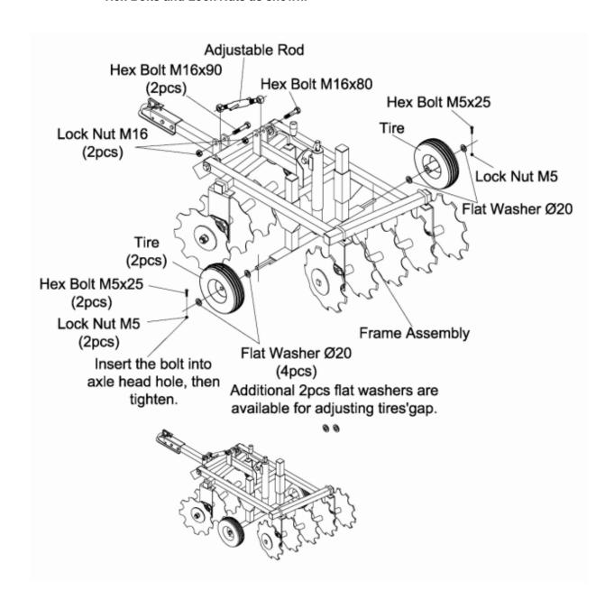
Step 6: There maybe some adjusting of the Hitch Tongue for the height of towing vehicle, this function can be performed by rotating handle on Adjusting Rod. Rotating the handle on the Mechanical Screw Jack will raise the tires up down.
