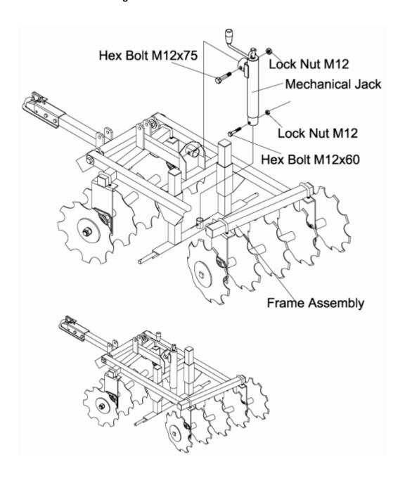
Step 5: Install Adjustable Rod to the Hitch Tongue and the Frame using the Hex Bolts and Lock Nuts as Shown.
