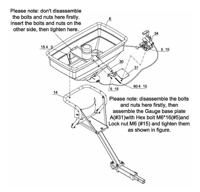
Step 7: Tighten all the nuts and bolts.
