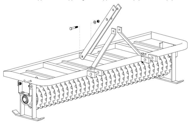
Step #5: Attach two Struts (4) to two Braces (5) using one Bolt (3), one Spacer (1), one Washer (10) and one Nut (15).
