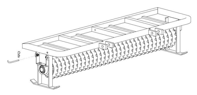
Step #3: Attach two Braces (5) to the Frame (6) using two Bolts (9), two Washers (10), and two Nuts (15)
