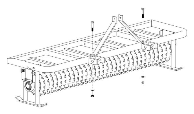
Step #4: Attach two Struts (4) to the Frame (6) using one Bolt (2), one Washer (10), and one Nut (15)
