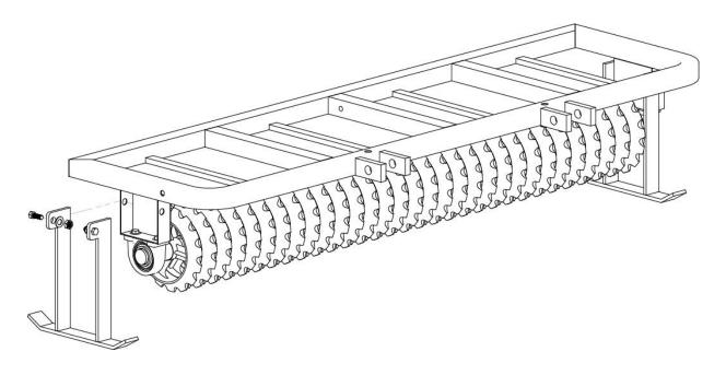
Step #2: Attach two Locking Pins (8) to the Frame (6) using two Clip Pins (7).
