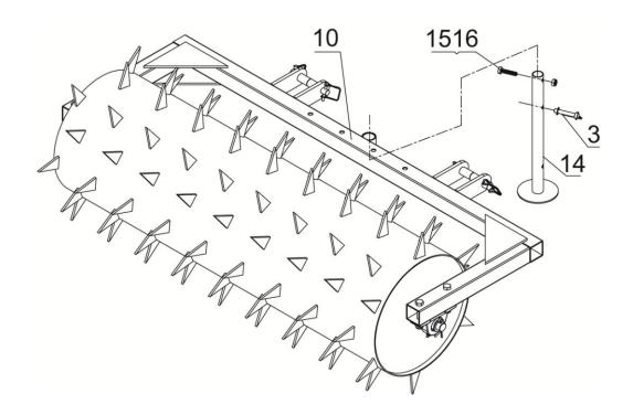
**Step 4:** Attach 3-point bracket (#5) to the frame (#10) using hex bolt M12x80 (#13), flat washer Ø12 (#6), and nylon lock nut M12 (#7).
