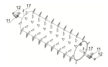
**Step 2:** Attach frame (#10) to the pillow block bearing (#11) using hex bolt M12x80 (#13), flat washer  $\emptyset$ 12 (#6), and nylon lock nut M12 (#7) to tighten, also tight the set screw in the collar make sure the shaft will not loose.
