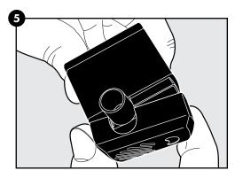
Next, remove the stator by placing your finger underneath the small lip, pulling it away from the pump.
