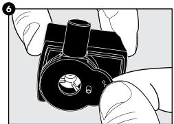
7. Use a fingernail to remove the impeller, which is held in place magnetically.
