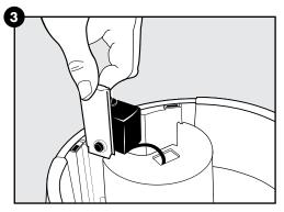
Next, pull the pump cord up through the opening until the pump is completely removed from the bowl piece. Remove the pump plate by simply pulling it away from the pump.
