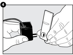
5. With your thumb and forefinger, gently squeeze on either side of the faceplate of the pump and pry it off. It may be necessary to insert a fingernail or other slim object into the seam of the faceplate.
