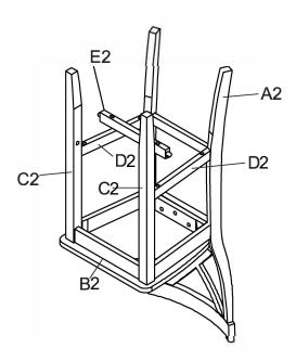
Step 4. Finger-tighten bolts (part #2), do not overtighten. Secure stretchers (parts D2 & E2) using screws (part #7) and phillips head screwdriver.
