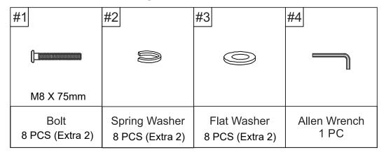
Step 1. Attach legs (part B) to table frame (part A) using bolts (part #1), spring washers (part #2), flat washers (part #3) and allen wrench (part #4).
