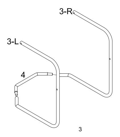
Step 3 Attach support legs (parts #3-L & 3-R) to chair back (part #1) using long bolts (part F), round plastic washers (part H), plastic washers (part G), flat washers (part C), nuts (part B), wrench (part D) and allen key (part E).
