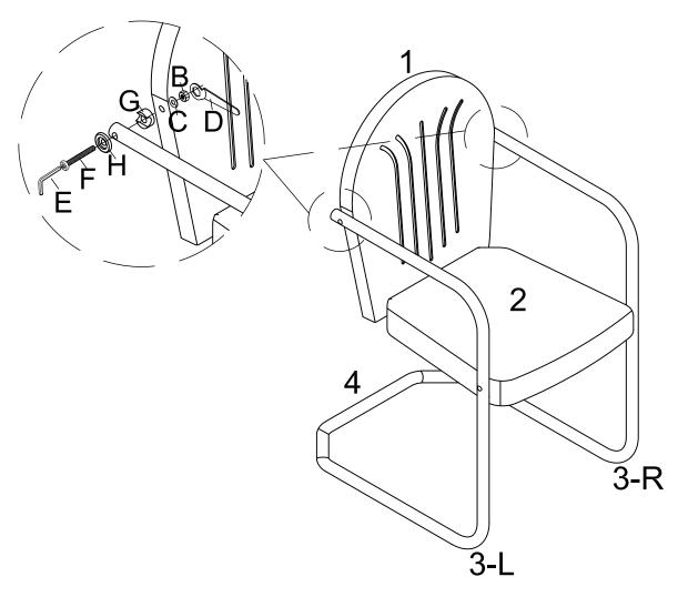
Step 4 Attach support legs (parts #3-L & 3-R) to chair seat (part #2) using long bolts (part F), round plastic washers (part H), plastic washers (part G), flat washers (part C), nuts (part B), wrench (part D) and allen key (part E).
