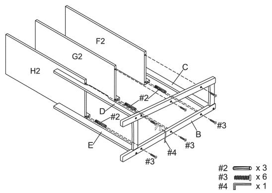
Step 3. Attach left side frame (part A) to back top rail (part C), top shelf (part F2), middle shelf (part G2), bottom shelf (part H2), front bottom rail (part D) and back bottom rail (part E) using wood dowels (part #2), allen bolts (part #3) and allen wrench (part #4).
