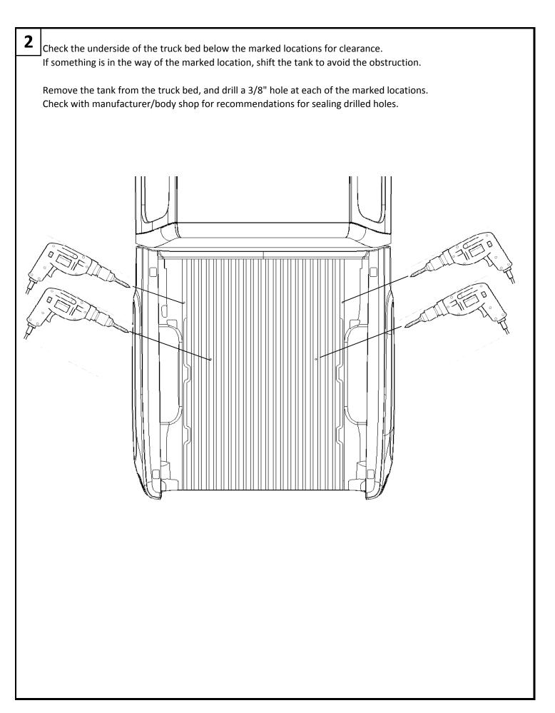
After drilling the holes, return the tank to the truck bed and align the tank mouting locations with the holes in the truck bed.
