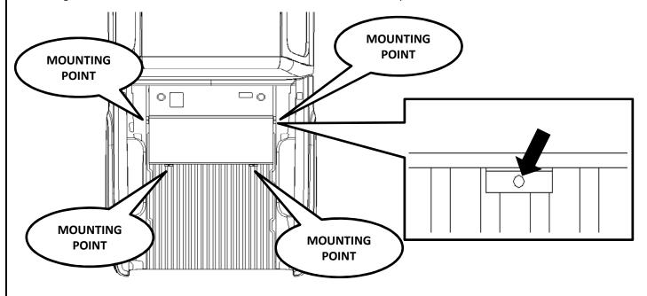
For rectangular shaped tanks there will be 2 mounting location on the front, and 2 on the back.
