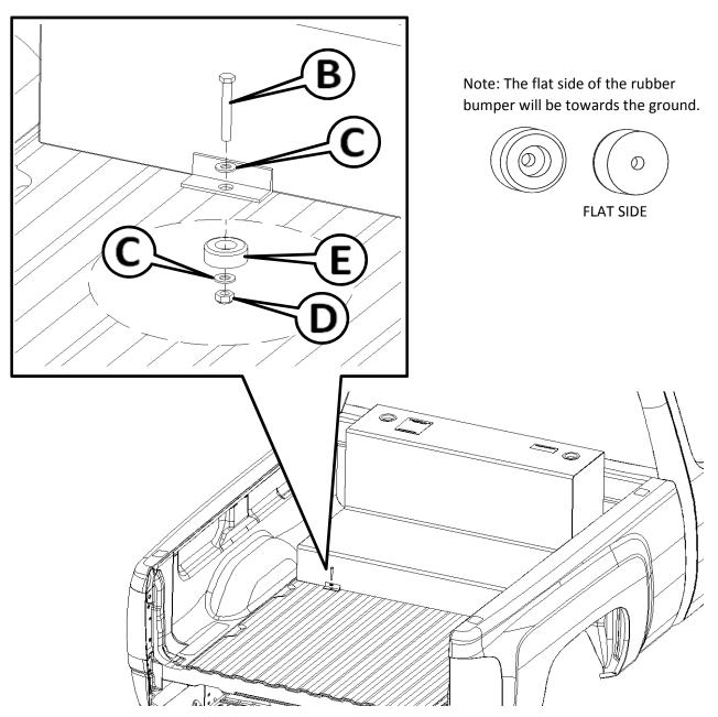
Tighten the nut and bolt using a 1/2" socket and wrench until the rubber bumper comes into contact with the underside of the truck bed. Grab the rubber bumper and try to rotate it around the bolt. If the rubber bumper can still rotate on the bolt, continue to tighten the nut until the rubber bumper can no longer be turned by hand. Once the rubber bumper can no longer be turned by hand, tighten the nut one additional 360 degree turn. Repeat this process for all four mounting locations.
