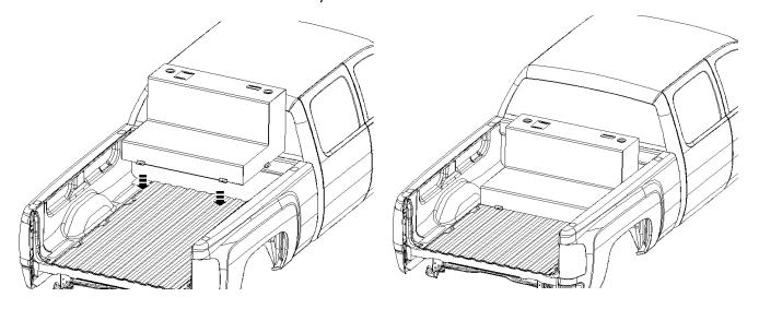
Using a marker, mark the hole location in the four tank attachment points.
