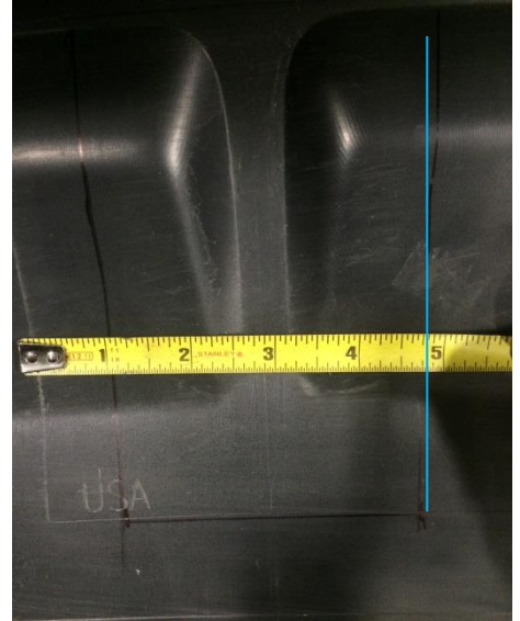
Scribe line 3 3/4" from previously scribed line, (4 3/4" from left side of USA section)
