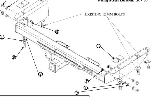
WARNING: DO NOT LUBRICATE THREADS, BOLT FAILURE MAY OCCUR DUE TO OVER TIGHTENING.
