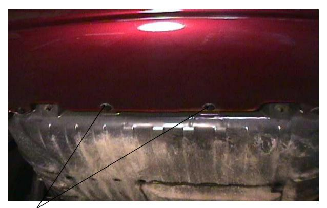
Remove these two plastic rivets to apply the cutting template.
