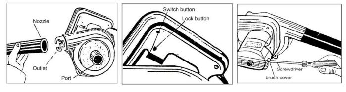
1. Attach the Nozzle to the Outlet. This will provide the necessary angle to the blower.
